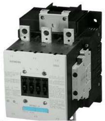
CONTACTOR, 75KW/400V/AC-3, AC(40...60HZ)/DC OPERATION UC 23...26V AUXIL. CONTACTS 2NO+2NC 3-POLE, SIZE S6 BAR CONNECTIONS CONVENTIONAL OPERATING MECHAN.
